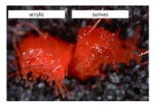
By way of example, here is a cross section of a spun-dyed acrylic and a yarn-dyed sunvas yarn.
