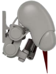
3) connection of the lower folding arm to the front profile
